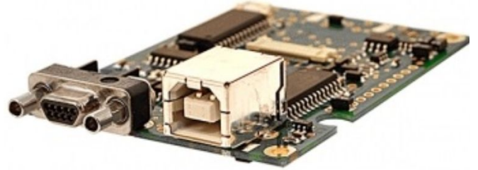
Figure 11: ATSAM21J18 Microcontroller Science Board
