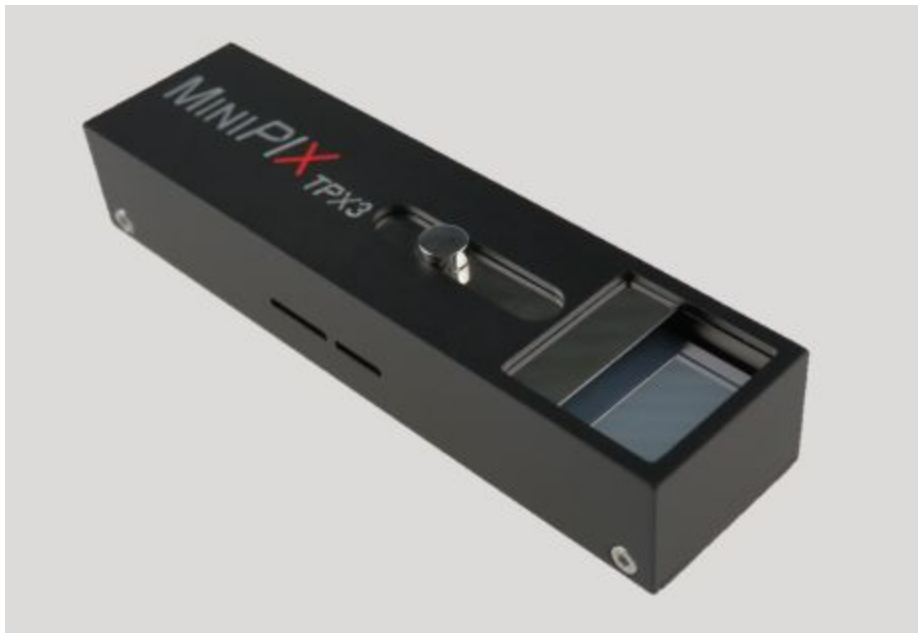
Figure 4: MiniPIX TPX3 Heavy Particle Detector
